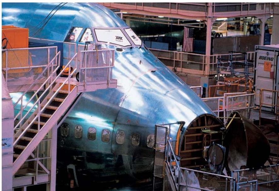
Aluminum is used in airplane construction.
