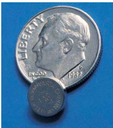
Batteries for electronic watches are, by necessity, very tiny.
