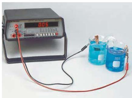
A concentration cell with 1.0 *M* Cu<sup>2+</sup> on the right and 0.010 *M* Cu<sup>2+</sup> on the left.
